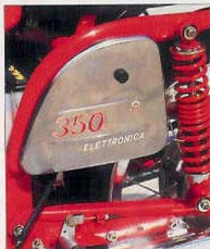
▲ Sidepanels announce flywheel triggered electronic ignition, introduced in 1972
